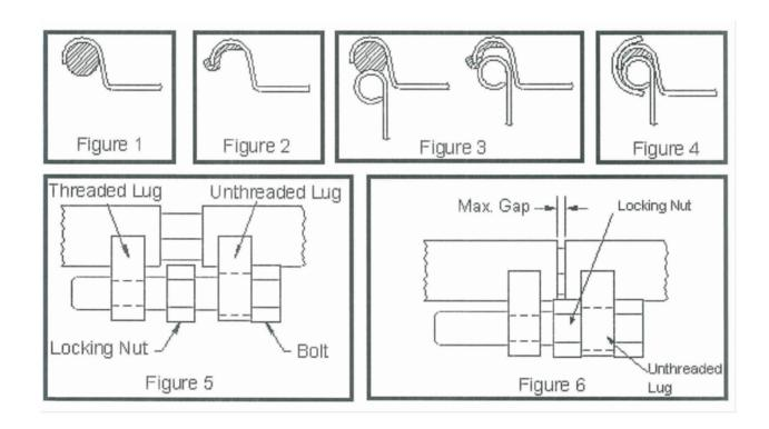
New Open Head New General Steel Drums With Out Locking Nut: 16 gauge body 15 – 20 ftlbs 12 gauge body 60 – 70 ftlbs.
