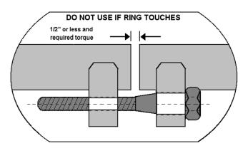
Steel Non Removable Head Drum Plug Torque Specifications
